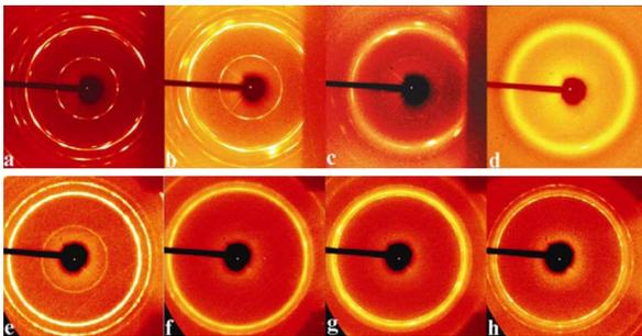
FIG. 3 (color online). X-ray diffraction images for:  $\text{Gd}_2\text{Ti}_2\text{O}_7$  at (a) 22.2 GPa, (b) 45.0 GPa, (c) 0 GPa (recovered sample and measured immediately), (d) 1 bar, 5 h after release of pressure.  $\text{Gd}_2\text{Zr}_2\text{O}_7$  at (e) 16.0, (f) 44.0, (g) 0 GPa (recovered sample and measured immediately) and (h) 1 bar, 10 h after releasing pressure.
