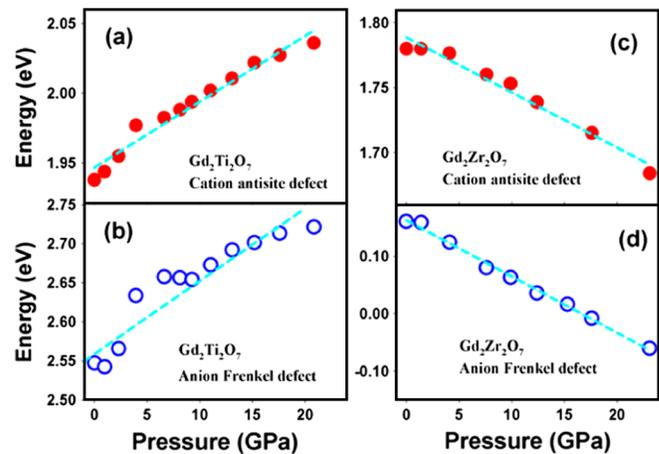
FIG. 4 (color online). Pressure dependence of the calculated formation energies of cation antisite defects and anion Frenkel defects in  $\text{Gd}_2\text{Ti}_2\text{O}_7$  and  $\text{Gd}_2\text{Zr}_2\text{O}_7$  pyrochlores. Dashed lines are only meant to guide the eyes.
