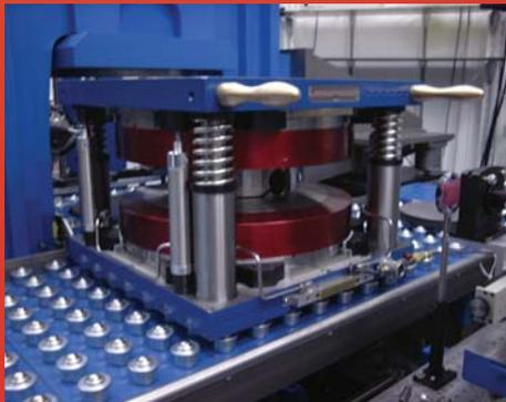
T-25 multi-anvil, high-pressure module installed in a 1000-ton press on GSECARS beamline at the Advanced Photon Source of the Argonne National Laboratory. Using this apparatus, pressures in excess of 25 GPa and temperatures over 2000 K can be obtained in samples of 1 cubic millimeter volume. Photo courtesy of Yanbin Wang, University of Chicago.
