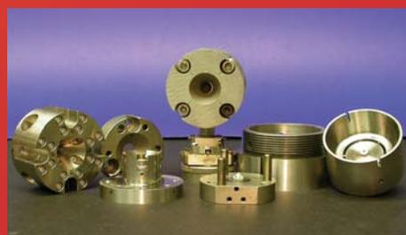
The natural diamond anvils in these different styles of high-pressure cells are approximately 1/4 carat in weight. Scaled-up devices would be used with the large synthetic diamonds of over 1 carat in weight to do a new generation of high-pressure experiments using larger samples. Photo courtesy of Dmitry Lakshatanov, Stanislav Sinogeikin, and Jay Bass, University of Illinois, Urbana-Champaign.
