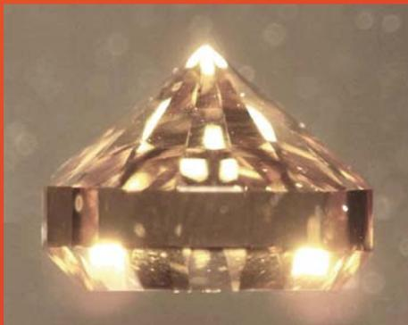
A research team at the Carnegie Institution of Washington and the Los Alamos National Laboratory has reported a major breakthrough in growing diamonds from chemical vapor deposition. They found that these high-pressure-temperature annealed crystals are the hardest diamonds ever tested. See Yan, C-s., H-k. Mao, W. Li, J. Qian, Y. Zhao, and R. J. Hemley, 2004, *Phys. Stat. Solidi*, (a) 201, R25.
