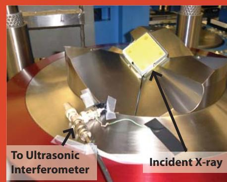
T-25 multi-anvil apparatus at the GSECARS beamline at the Advanced Photon Source, Argonne National Laboratory, as used for ultrasonic velocity measurements at the pressures and temperatures characteristic of Earth's transition zone. Photo courtesy of Yanbin Wang, University of Chicago, and Baosheng Li, Stony Brook University.
