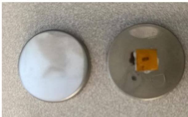
Figure 1. Normal coin cell shell (left) and modified coin cell shell with Laser Miller (right).
