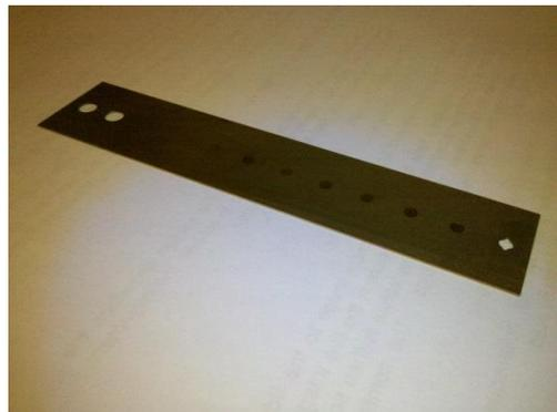
Figure 2-Finished collimator mask assembly
