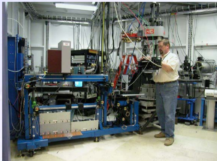
Installation of monochromatic side-station in the X17B2 hutch of the NSLS
