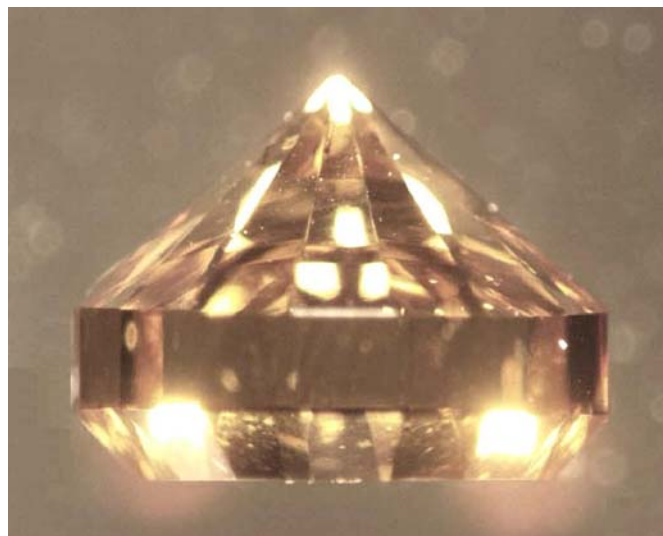
Modified brilliant cut single-crystal diamond grown by chemical vapor deposition (CVD). About 2.5 mm high, this crystal was grown in one day at Carnegie Institution. The very bottom (table) of the crystal is a type Ib seed; hence the yellow tint is due to internal reflection (the CVD diamond is transparent) (Yan et al. 2004).
