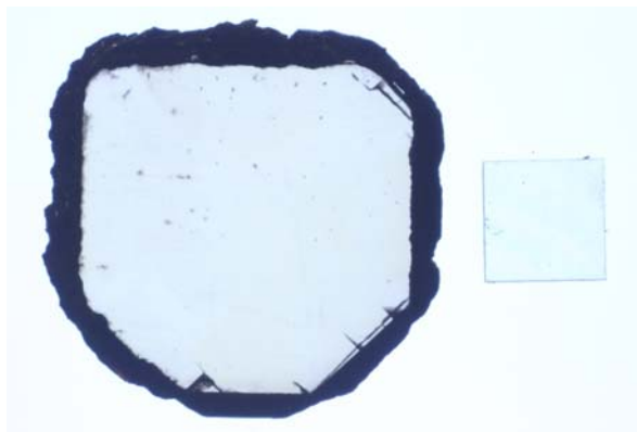
A 5 x 5 x 0.5 mm single crystal plate grown in 5 hours at Carnegie; right: a HPHT plate available from De-Beers (Element Six).
