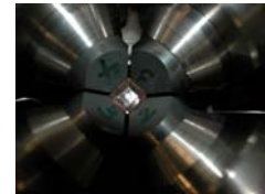
P and S wave velocity of pyrolyte model through acoustic measurements at high P and T (Li et al. Science 1998)
