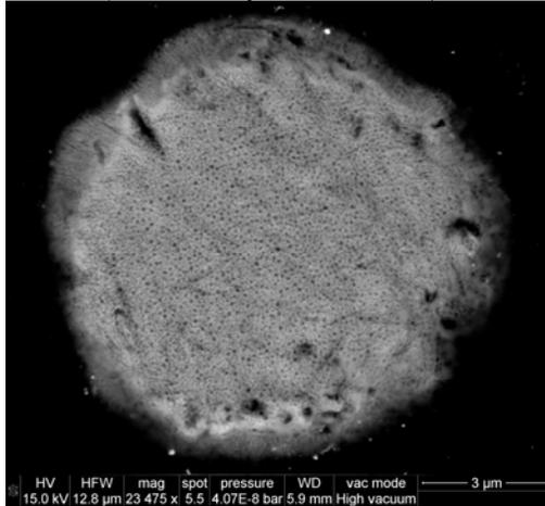
Fig. 1: Backscattered electron image of a laser heated spot in an Fe-Si-O sample recovered from 60 GPa and 4900 K. X-ray diffraction data indicates that at these conditions the sample was completely molten.
