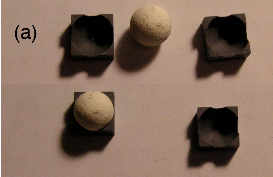
Fig. 2. Custom cell of mullite sphere and pyrophyllite cradles for D-DIA apparatus fabricated in multi-anvil cell development program at the Arizona State University by Kurt Leinenweber and colleagues for deformation experiments at the X17B2 beamline of the National Synchrotron Light Source.
